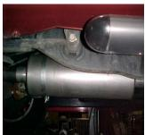
LAY OUT THE GIBSON EXHAUST ON THE FLOOR AND COMPARE PART #'S TO THE DRAWING. TO REMOVE YOUR FACTORY EXHAUST UN-BOLT YOUR TAILPIPE AT THE 2-BOLT FLANGE LOCATED BEHIND YOUR STOCK MUFFLER USE WD-40 TO AID YOU IN REMOVAL OF HANGERS FROM RUBBER GROMMETS.
