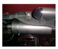
INSTALL MUFFLER # C ONTO YOUR RESONATOR#B 1 ½" –2". USE CLAMP # I TO SECURE MUFFLER TO THE PIPE, DO NOT TIGHTEN.
