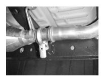
REMOVE STOCK EXHAUST BY UN-CLAMPING THE STOCK CLAMP AT THE HEADPIPE. BE CAREFUL NOT TO DAMAGE THIS CLAMP BECAUSE YOU NEED TO RE-USE IT. ONCE IT IS UN-CLAMPED, YOU WILL BE ABLE TO PULL THE STOCK EXHAUST OFF THE VEHICLE. MAKE SURE ALL FACTORY RUBBER GROMMETS ARE STILL IN FACTORY LOCATION. USE WD-40 TO AID YOU IN REMOVAL OF THE HANGERS
