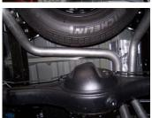
9. Install driver side overaxle tailpipe #G onto extension pipe, use clamp #J to secure pipe. Do not tighten. Insert welded hanger into rubber grommet.
