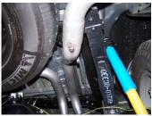
7. Install the passenger side overaxle tailpipe #F to the extension pipe. Use clamp #J to secure. Do not tighten. Insert welded hanger into rubber grommet.
