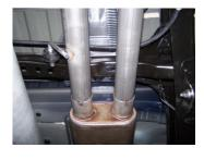
6. Install extension pipe #D into muffler. Use clamp #J to secure. Do not tighten. Next install driver side extension pipe #E into muffler using clamp #J to secure. Do not tighten. Insert welded hanger into rubber grommet.
