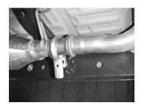
REMOVE STOCK EXHAUST BY UN-CLAMPING THE STOCK CLAMP AT THE HEADPIPE. BE CAREFUL NOT TO DAMAGE THIS CLAMP BECAUSE YOU NEED TO RE-USE IT. ONCE IT IS UN-CLAMPED, YOU WILL BE ABLE TO PULL THE STOCK EXHAUST OFF THE VEHICLE. MAKE SURE ALL FACTORY RUBBER GROMMETS ARE STILL IN FACTORY LOCATION. USE WD-40 TO AID YOU IN REMOVAL OF THE HANGERS FORM THE GROMMETS.
