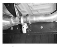
LAY OUT THE GIBSON EXHAUST ON THE FLOOR SO IT LOOKS LIKE THE DRAWING AND COMPARE PART NUMBERS. DISCONNECT THE FACTORY CLAMP IN FRONT OF THE STOCK MUFFLER AND REMOVE THE FACTORY EXHAUST. DO NOT DAMAGE THE FACTORY CLAMP. YOU WILL RE-USE IT. LEAVE
