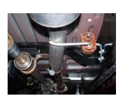
TO REMOVE YOUR STOCK REMOVE IT FROM THE CL, LOCATED JUST IN FRONT MUFFLER REMOVE HANGE RUBBER GROMMETS BY PU EXHAUST TOWARDS THE THE VEHICLE, USE WD-40 REMOVAL, LEAVE GROMME PLACE.
