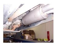
MAKE SURE YOU AT LEAST A 1" CLEARANCE AWAY FROM ALL BRAKE LINES, FUEL LINES, SHOCKS, TIRES, ETC. 2004 FORD F-150 ECSB 5.4L SUPERTRUCK
