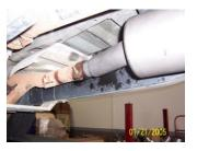
NEXT, INSTALL MUFFLER ASSEMBLY # A INTO STOCK HEADPIPE. DO NOT TIGHTEN, USE YOUR FACTORY CLAMP TO SECURE.
