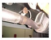
**1.** To remove the stock exhaust remove it from the clamp located in front of the stock muffler. Disengage the welded hangers using WD-40 from the OEM rubber grommets. Do not damage or remove the rubber grommets as you will re-use them to mount your new system. Now, cut off tailpipe and remove exhaust.
