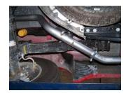
**5.** Install the passenger side overaxle tailpipe #C into the muffler  $1\frac{1}{2}$ "-2". Use clamp #Hto secure tailpipe to muffler. DO NOT TIGHTEN. Insert hanger into rubber grommet.
