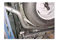
Next, install drivers side tailpipe # C into muffler 1-1/2" to 2" route between spare tire and shocks use clamp # G to secure, do not tighten. Next install exit pipe #M onto tail pipe. Use clamp #G to secure, do not tighten
