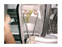
Next install both tailpipe hangers into rubber grommets. Then adjust it to your liking.
