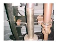
Install welded headpipe hanger into rubber grommet.
