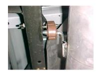
Install welded muffler hanger into rubber grommets.
