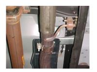
Lay out the exhaust on the floor so it looks like the drawing and compare parts with manual. To remove the stock exhaust using WD-40 take all hangers out of grommets.
