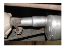
SLIDE INLET OF MUFFLER ASSEMBLY #A ONTO CATALYTIC CONVERTER. USE CLAMP #B TO SECURE. DO NOT TIGHTEN.
