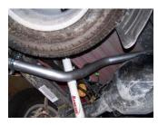
**7.** Install the driverside overaxle tailpipe #D into the muffler 1½-2". Use clamp #H to secure. DO NOT TIGHTEN. Rotate until it meets with metal hanger, use clamp #H to hold pipe. DO NOT TIGHTEN.
