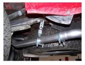
**6.** Install metal hanger #I into hole located approximately 19" from the rear of the frame in the second hole from top. Use bolt kit #J to secure. DO NOT TIGHTEN.
