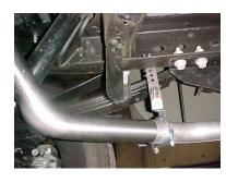
INSTALL PASSENGER SIDE OVERAXLE PIPE #C INTO MUFLER 1 <sup>1</sup>/<sub>2</sub>" TO 2". USE CLAMP # I TO SECURE. DO NOT TIGHTEN. ROTATE UNTIL PIPE TOUCHES HANGER. USE CLAMP #I TO HOLD PIPE TO HANGER #J. DO NOT TIGHTEN.
