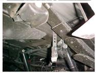
NEXT, INSTALL DRIVERS SIDE OVERAXLE PIPE #D INTO MUFFLER 1 <sup>1</sup>/<sub>2</sub>" TO 2". USE CLAMP #I TO SECURE PIPE TO MUFFLER. DO NOT TIGHTEN. ROTATE PIPE UNTIL IT TOUCHES HANGER. USE CLAMP #I TO HOLD PIPE TO HANGER DO NOT TIGHTEN.
