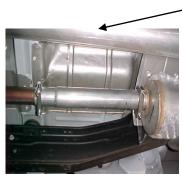
INSTALL NEW HEADPIPE #A AND ATTACH USING CLAMP #G TO FACTORY PIPE.
