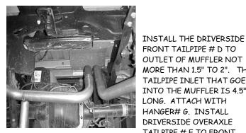
FRONT TAILPIPE # D TO **OUTLET OF MUFFLER NOT** MORE THAN 1.5" TO 2". THE TAILPIPE INLET THAT GOES INTO THE MUFFLER IS 4.5" LONG. ATTACH WITH HANGER# G. INSTALL DRIVERSIDE OVERAXLE TAILPIPE # E TO FRONT DRIVERSIDE TAILPIPE, THIS PART HAS A SWEDGE UP ON IT. ATTACH USING CLAMP # G. INSTALL PASSENGER OVERAXLE TAILPIPE TO THE **OUTLET OF THE MUFFLER** NOT MORE THAN 1.5" TO 2". THE TAILPIPE INLET THAT GOES INTO THE MUFFLER IS 4.5" LONG AND ATTACH WITH CLAMP # G. DO NOT TIGHTEN.
