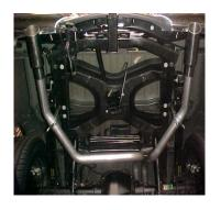
INTSTALL EXIT PIPES # F TO THE OVERAXLE TAILPIPES USE CLAMP # G TO SECURE USE ZIP TIES FOR BRAKE AND HOSE LINES TO KFFP AWAY FROM PIPES, NOW FIRMLY TIGHTEN ALL BOLTS, CLAMPS AND HANGERS. INSTALL STAINLESS TIPS.
