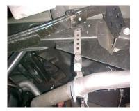
ON DRIVER SIDE MEASURE 17-1/2" FROM THE REAR OF THE FRAME FORWARD. USE HANGER # I. USE THE TOP HOLE OF THIS HANGER. USE HARDWARE PROVIDED. REPEAT FOR PASS. SIDE.
