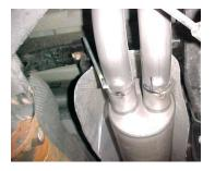
INSTALL DRIVERS SIDE TAILPIPE # D INTO MUFFLER 1 ½" TO 2". INSERT HANGERS INTO RUBBER GROMMETS, USE CLAMP # G TO SECURE PIPE TO MUFFLER. DO NOT TIGHTEN. THE TAB ON THIS PIPE SHOULD GO ON BOTTOM OF PASSENGER SIDE PIPE USE BOLT KIT # H TO SECURE TOGETHER.
