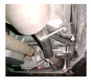
INSTALL HEADPIPE # A INTO STOCK PIPE. THE END OF THE PIPE SHOULD BE AT THE 12 O'CLOCK POSITION, ATTACH WITH FACTORY CLAMP TO HEADPIPE. DO NOT TIGHTEN.
