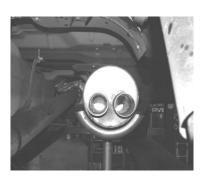
INSTALL MUFFLER INLET ONTO HEADPIPE 1-1/2" TO 2" AND ATTACH USING CLAMP #H. DO NOT TIGHTEN, USE A JACKSTAND TO SUPPORT MUFFLER. OUTLETS SHOULD BE ON THE BOTTOM.
