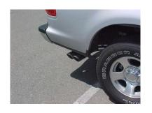
INSTALL THE DRIVERSIDE FRONT TAILPIPE #C TO OUTLET OF MUFFLER AND ATTACH WITH HANGER #K AND INSERT INTO WELDED RUBBER HANGER. INSTALL DRIVERSIDE OVERAXLE TAILPIPE #D TO FRONT DRIVERSIDE TAILPIPE AND ATTACH USING CLAMP #J TO FRONT PIPE. INSTALL PASSENGER SIDE FRONT TAILPIPE #E TO OUTLET OF MUFFLER AND ATTACH WITH CLAMP #J.
