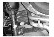
NEXT INSTALL DRIVERS OVER AXLE PIPE # D INTO MUFFLER 1½ TO 2".USE CLAMP # F TO SECURE PIPE TO MUFFLER. DO NOT TIGHTEN. USE BOLT KIT # H TO SECURE PIPES TOGETHER. DRIVERSIDE TAB WILL BE ON THE BOTTOM.
