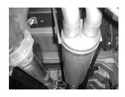
SLIP MUFFLER #B THROUGH BAND CLAMP THEN ONTO THE HEADPIPE 1 ½" TO 2". THE OUTLETS WILL BE LEVEL. USE CLAMP #G TO SECURE MUFFLER TO HEADPIPE. DO NOT TIGHTEN.
