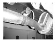
TO REMOVE YOUR STOCK EXHAUST, UNBOLT AND REMOVE THE CLAMP LOCATED JUST IN FRONT OF THE MUFFLER. FOR EASIER REMOVAL OF THE FACTORY EXHAUST, CUT OFF THE STOCK TAILPIPE JUST BEHIND THE MUFFLER AND REMOVE. LEAVE ALL RUBBER GROMMETS ON THE HANGERS. USE WD-40 TO AID IN REMOVAL OF EXHAUST AND HANGERS.
