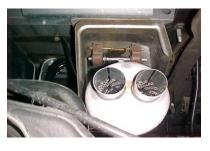
SLIP MUFFLER #B THROUGH BAND CLAMP THEN ONTO THE HEADPIPE 1 ½" TO 2". THE OUTLETS WILL BE ON THE TOP. USE CLAMP #F TO SECURE MUFFLER TO HEADPIPE. DO NOT TIGHTEN.
