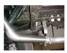
INSTALL PASSENGER SIDE OVERAXLE PIPE #C INTO MUFLER 1 ½" TO 2" USE CLAMP # T T
