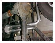
NEXT, INSTALL DRIVERS SIDE TAILPIPE # D INTO MUFFLER 1 1/2" -2". USE CLAMP # J TO SECURE PIPE INTO MUFFLER, DO NOT TIGHTEN. ROTATE PIPE UNTIL IT MAKES CONTACT WITH HANGER # K USE CLAMP # J TO HOLD PIPE UP. NEXT, INSTALL EXIT PIPES # F ONTO TAILPIPE, DO NOT TIGHTEN, REPEAT THIS STEP FOR THE PASS. SIDE, USING TAILPIPE # E.
