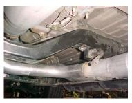
INSTALL Y-PIPE # A & O ONTO STOCK FLANGES USE YOUR STOCK HARDWARE TO SECURE INSERT WELDED HANGER INTO RUBBER GROMMET, DO NOT TIGHTEN.
