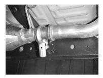
REMOVE STOCK EXHAUST BY UN-CLAMPING THE STOCK CLAMP AT THE HEADPIPE. BE CAREFUL NOT TO DAMAGE THIS CLAMP BECAUSE YOU NEED TO RE-USE IT. ONCE IT IS UN-CLAMPED, YOU WILL BE ABLE TO PULL THE STOCK EXHAUST OFF THE VEHICLE. MAKE SURE ALL FACTORY RUBBER GROMMETS ARE STILL IN FACTORY LOCATION. USE WD-40 TO AID YOU IN REMOVAL OF THE HANGERS
