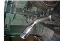
INSTALL EXIT PIPES # E ONTO TAILPIPES USE CLAMP # I TO SECURE PIPES TOGETHER CLAMP ON, DRIVERS SIDE WILL HOOK UP TO THE REAR HANGER TO HOLD PIPES UP.
