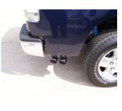
9. Install stainless steel tips. Clamp down. When you have everything in place, firmly tighten all bolts and clamps down securely. Use stainless steel cleaner and a Scotch Brite pad weekly to prevent tip from discoloration. Inspect all fasteners after 25-50 miles of operation and re-tighten as necessary.
