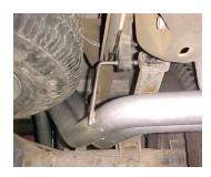
INSTALL PASSENGER OVERAXLE TAILPIPE #C. INSERT WELDED HANGER INTO RUBBER GROMMET. DO NOT TIGHTEN. ATTACH TAILPIPE TO THE MUFFLER USING CLAMP # F. USE BOLT KIT # I TO ATTACH BOTH OVERAXLE PIPES TOGETHER. THE SPARE TIRE ON SOME VEHICLES MAY NEED TO BE LOOSENED AND PULLED TO THE DRIVERSIDE FOR BETTER CLEARANCE.
