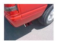
INSTALL THE STAINLESS TIPS. NOW GO BACK AND START AT THE FRONT AND TIGHTEN ALL CLAMPS AND HANGERS.
