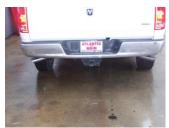
**9.** Install stainless steel tips #F. Clamp down. When you have everything in place, firmly tighten all bolts and clamps down securely. Use stainless steel cleaner and a Scotch Brite pad weekly to prevent tip from discoloration.
