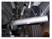
**5.** Install the passenger side overaxle tailpipe #C into the muffler 1½"-2". Use clamp #G to secure tailpipe to muffler. DO NOT TIGHTEN. Insert welded hanger into rubber grommet.
