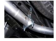
**8.** Install exit pipes #E onto tailpipe and secure with clamp #H. DO NOT TIGHTEN.
