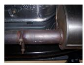
**1.** To remove the stock exhaust remove it from in front of the stock muffler. DO NOT REMOVE STOCK HEADPIPE. Disengage the welded hangers using WD-40 from the OEM rubber grommets. Do not damage or remove the rubber grommets as you will re-use them
