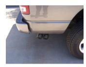
**11.** Install stainless steel tips #E. Clamp down. When you have everything in place, firmly tighten all bolts and clamps down securely. Use stainless steel cleaner and a Scotch Brite pad weekly to prevent tip from discoloration.
