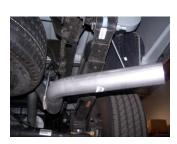
**5.** Install the passenger side overaxle tailpipe #D into the muffler 1½"-2". Use clamp #F to secure tailpipe to muffler. DO NOT TIGHTEN. Insert welded hanger into rubber grommet.
