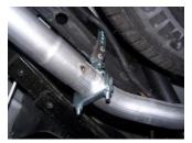
7. Install exit pipes #E, use clamps #G to secure to tailpipes. DO NOT TIGHTEN. Roll pipes until you have the angle you desire.
