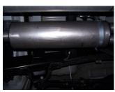
3. Install muffler #B onto head pipe #A 1½"-2" with the louvers facing towards the converter. Use a jack stand to support the muffler. Use clamp #H to secure the muffler to the headpipe. Slide band clamp #I onto muffler and insert welded hangers into rubber grommets. Attach with bolt kit #K. DO NOT TIGHTEN. Muffler inlet is looking into the louvers.
