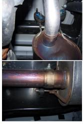
1. To remove the stock exhaust un-clamp the tailpipe just after the stock muffler. Then un-clamp the stock muffler. Leave all rubber grommets in place. Use WD-40 to
