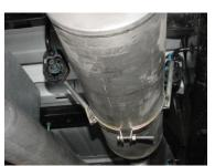
INSTALL HEADPIPE #A ONTO YOUR EXISTING STOCK FRONT PIPE AND SECURE WITH CLAMP #G. USE A JACKSTAND TO SUPPORT THE CONVERTER. INSERT WELDED HANGER INTO RUBBER GROMMET.
