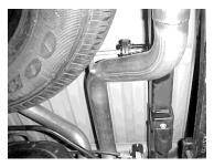
INSTALL THE PASSENGER SIDE TAILPIPE #C INTO THE MUFFLER AT LEAST 1-1/2" TO 2". BE SURE TO INSERT THE WELDED HANGER INTO THE RUBBER GROMMET. USE 2-1/2"CLAMP #J TO SECURE THE PIPE TO THE MUFFLER. DO NOT TIGHTEN.
