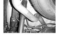
INSTALL THE DRIVER SIDE TAILPIPE #D INTO THE MUFFLER AND LEAST 1-1/2" TO 2". THIS PIPE WILL ROUTE OVER THE AXLE, BETWEEN THE SHOCK AND TIRE. USE CLAMP #J TO SECURE THE PIPE TO THE MUFFLER. **DO NOT TIGHTEN.** THEN, INSERT THE HANGERS INTO THE RUBBER GROMMETS.
