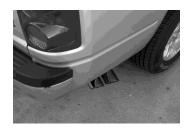
Install the stainless tips. Clamp down. To clean your stainless tips use any stainless cleaner. Now go back and tighten all clamps, nuts and bolts. Start from the front and work back.
