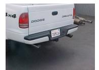
INSTALL YOUR STAINLESS STEEL TIPS. NOW GO BACK AND TIGHTEN ALL CLAMPS, NUTS AND BOLTS STARTING FROM THE FRONT AND WORK YOUR WAY BACK.
