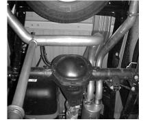
INSTALL PASSENGER SIDE OVERAXLE PIPE #D AND ATTACH TO MUFFLER USING CLAMP # F. INSERT HANGER INTO RUBBER GROMMET.
