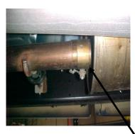
DO NOT REMOVE THE EXTENSION PIPE BETWEEN THE MUFFLER AND THE CONVERTER.
