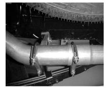
ATTACH EXIT PIPES # D TO OVERAXLE PIPES AND ATTACH WITH CLAMP # E.
