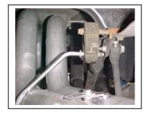
Install the driver side over axle tailpipe # C into the muffler. 1-1/2 TO 2". iInsert welded hanger into rubber grommet. Use clamp #e to secure tailpipe to muffler. Do not tighten.
