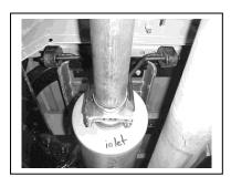
Install muffler onto head pipe # A 1-1/2" to 2" with the louvers facing towards the converter. Use a jack stand to support the muffler. Use clamp to secure the muffler to the head pipe. Do not tighten. Muffler inlet is looking into the louvers.
