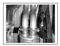
Install passenger side over axle tailpipe # B into muffler 1-1/2" – 2" and attach using clamp # E .
