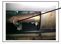
To remove the stock exhaust un-clamp it just in front of the muffler. You may need to heat it up for easier removal. Leave all rubber grommets in place. Use WD-40 to aid in removal of exhaust and the hangers.
