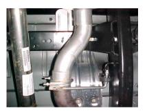
**INSTALL HEADPIPE #A,** YOU WILL NEED TO LINE UP THE TWO NOTCHES. **USE HANGER #J TO** SECURE HEADPIPE TO THE STOCK PIPE. DO NOT TIGHTEN. INSERT HANGER INTO RUBBER GROMMET.
