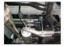
**INSTALL MUFFLER ASSEMBLY #A ONTO** STOCK PIPE 1-1/2" TO 2". SLIDE WELDED HANGERS INTO RUBBER **GROMMETS YOU** MAY NEED TO ADJUST WELDED HANGERS TO FIT INTO YOUR GROMMETS. USE A JACKSTAND TO SUPPORT YOUR MUFFLER. USE CLAMP #B TO SECURE IT TO YOUR HEADPIPE. DO NOT TIGHTEN
