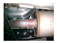
YOU MAY NEED TO HEAT IT UP FOR EASIER REMOVAL. LEAVE ALL RUBBER GROMMETS IN PLACE. USE WD-40 FOR REMOVAL OF HANGERS.
