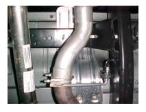
INSTALL HEADPIPE #A, YOU WILL NEED TO LINE UP THE TWO NOTCHES. USE HANGER #J TO SECURE HEADPIPE TO THE STOCK PIPE. DO NOT TIGHTEN. INSERT HANGER INTO RUBBER GROMMET.
