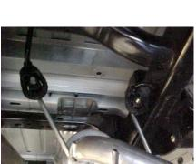
**INSTALL MUFFLER** ASSEMBLY #A ONTO HEADPIPE 1-1/2" TO 2". SLIDE WELDED HANGERS INTO RUBBER GROMMETS YOU MAY NEED TO **ADJUST WELDED** HANGERS TO FIT INTO YOUR GROMMETS. USE A JACKSTAND TO SUPPORT YOUR MUFFLER. USE CLAMP #B TO SECURE IT TO YOUR HEADPIPE. DO NOT TIGHTEN.
