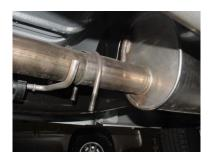
TO REMOVE STOCK **EXHAUST UNCLAMP IT** FROM THE CLAMP LOCATED JUST IN FRONT OF YOUR STOCK MUFFLER. YOU MAY NEED TO HEAT IT UP WITH A TORCH TO REMOVE IT. NOW CUT OFF YOUR STOCK TAILPIPE JUST BEHIND THE MUFFLER AND REMOVE.LEAVE ALL **RUBBER GROMMETS** ON THE HANGER. USE WD-40 TO AID IN **REMOVAL OF EXHAUST AND** HANGERS.
