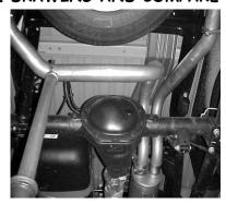
INSTALL PASSENGER SIDE OVERAXLE PIPE #D AND ATTACH TO MUFFLER USING CLAMP # F. ATTACH HANGER # H AND CLAMP #F TO OVERAXLE TAILPIPE.
