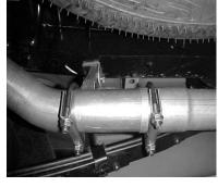
ATTACH EXIT PIPES # D TO OVERAXLE PIPES AND ATTACH WITH CLAMP # F
