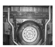
1-1/2" TO 2" FROM BEHIND THE AXLE AND CONNECT TO THE MUFFLER AND ATTACH WITH CLAMP **#F.** INSERT WELDED HANGER INTO RUBBER GROMMET. ATTACH HANGER #H USING CLAMP #F TO TAILPIPE. REPEAT THE SAME FOR THE DRIVERSIDE OVERAXLE TAILPILPE # D. IF YOU CAN NOT GET THE PASSENGER TAILPIPE TO CLEAR REMOVE SPARE TIRE AND ROTATE THE MUFFLER TOWARDS THE DRIVERSIDE AND ALIGN TAILPIPES AWAY FROM THE SHOCK.
