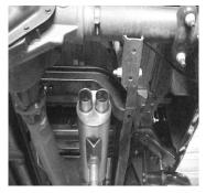
CONNECT MUFFLER WITH THE INLET TOWARDS THE CONVERTER. MAKE SURE REAR OF MUFFLER OUTLETS SIT AT 3 AND 9 O'CLOCK. ALLOW A MINIMUM OF 1 ½" TO SLIDE OVER THE HEADPIPE. USE A JACKSTAND TO SUPPORT THE MUFFLER AND CONNECT CLAMP # G. DO NOT TIGHTEN.
