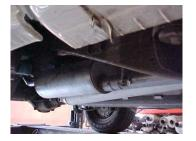
Install the driver side over axle tailpipe # D into the muffler. Use clamp # F to secure tailpipe to muffler. Do not tighten. Insert hanger into rubber grommet.
