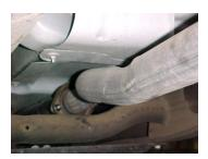
Lay out the exhaust on the floor so it looks like the drawing and compare parts with manual. To remove the stock exhaust un-bolt it from the flange located in front of the muffler. You will re-use your stock hardware. Leave all rubber grommets in place. Use WD-40 to aid in removal of exhaust and the hangers. Cut your stock tailpipe off just
