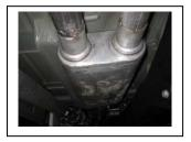
5. Install muffler #B onto head pipe #A 1½"-2" with the louvers facing towards the converter. Use a jack stand to support the muffler. Use clamp #f to secure the muffler to the head pipe. Do not tighten. Muffler inlet is looking into the louvers.
