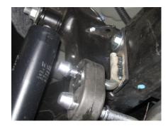
5.Next install drivers side rear hanger and gommet with bolt kit provided see picture the hanger goes on the outside of the frame and bolts through the whole frame
