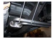
4. Rotate the muffler assembly until the outlets are level.
