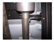
4. Slide muffler #B over support the muffler. Use clamp #E to secure the muffler to the
