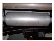
headpipe 1.5-2" with the louvers facing towards the converter. Use a jack stand to headpipe. Do not tighten. Muffler inlet is looking into the louvers.
