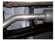
4. Slide muffler #B over headpipe 1.5-2" with the louvers facing towards the converter. Use a jack stand to support the muffler. Use clamp #F to secure the muffler to the headpipe. Do not tighten. Muffler inlet is looking into the louvers.
