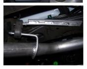
**8.** Install the exit pipes #E and #F. Use clamp #H to secure exit pipes to tailpipes. DO NOT TIGHTEN.
