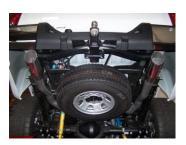
8. Install exit pipes #E. Use clamps #H to secure tailpipes. Do not tighten. May need to trim the exit pipes to best fit your vehicle.
